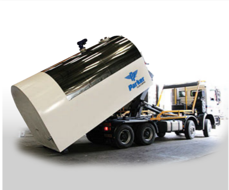
Loading 18,000 litre Hook Lift Bunded Tank for re-location
